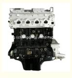
4G15 Complete Motor Changan OUSHANG 4G15 Engine Long Block Engine Assembly
